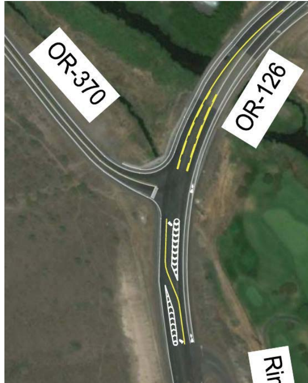
Figure 4. Applicant's suggested removal of the uphill passing lanes and replacement of the back-to-back left-turn lanes with side-by-side turn lanes.
