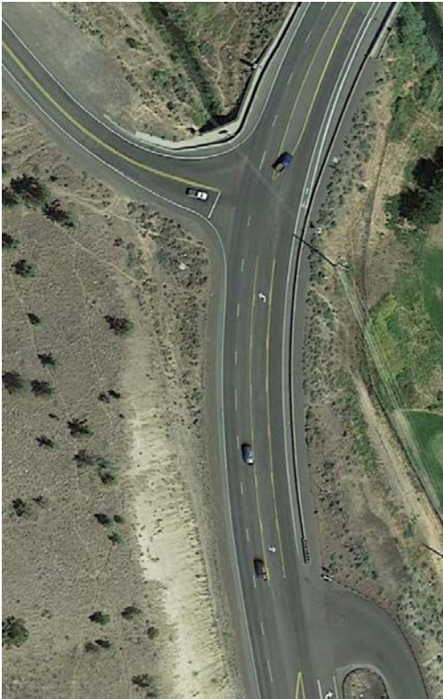
Figure 3. Current intersection configuration with back-to-back left-turns between OR 370 and Rimrock Drive.
