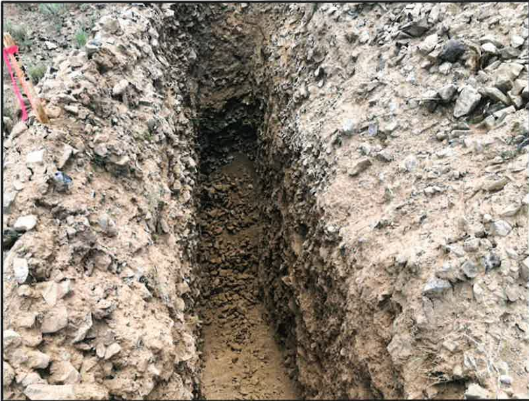
TP-08 trench profile. Note main cobble unit.
